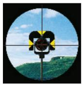
Gone are the days when you had to spend a lot of time aiming at the target to be measured. Today, TPS700 instruments perform this task with automatic target recognition (ATR).
