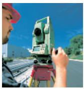
Gone are the times when targets had to be aimed at manually. The TPS 700 performs this and other standard processes with its intelligent software and motorized drives.
