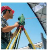
Gone are the times when hard to access targets could only be measured with a lot of effort. Now there are the TPS700 instruments featuring reflectorless distance measurement.
